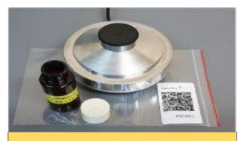
Short-term measurement device of 3-4 days average Radon Concentration Level (RCL)
